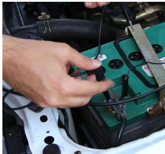
Interface probe to the lizard clamp connection
