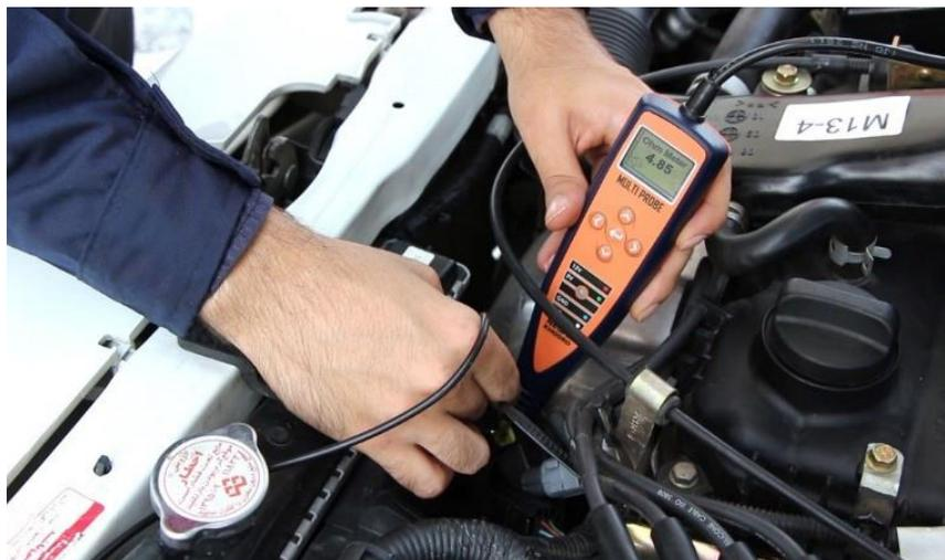
Oxygen sensor ohmic test
