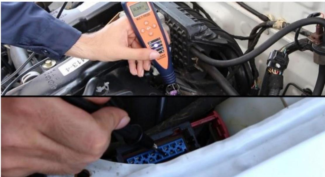
Testing the injector supply to double relay
