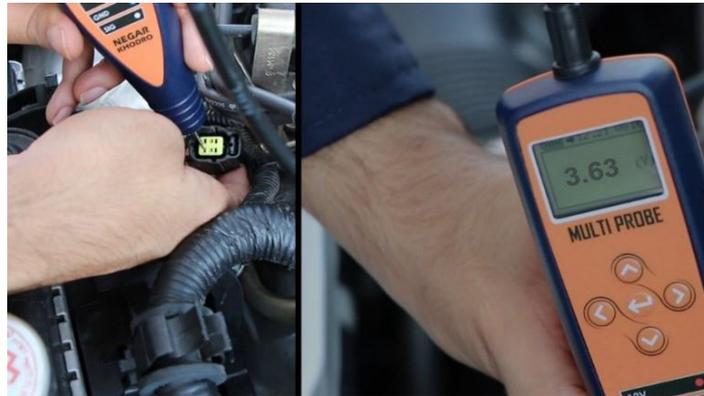
oxygen sensor test
