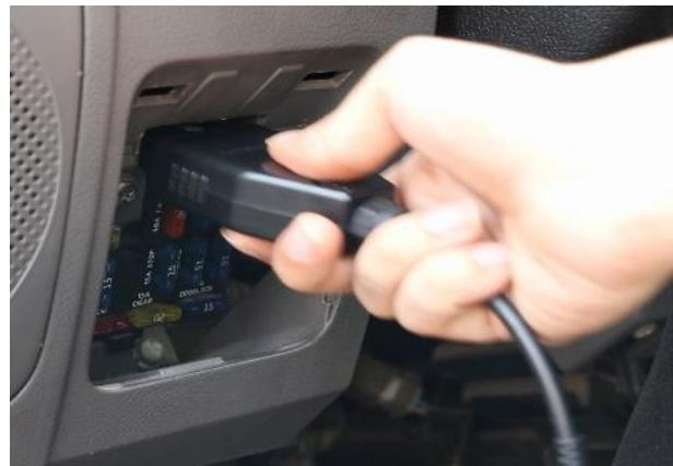
Connection to the car OBD socket and flashing ECU
