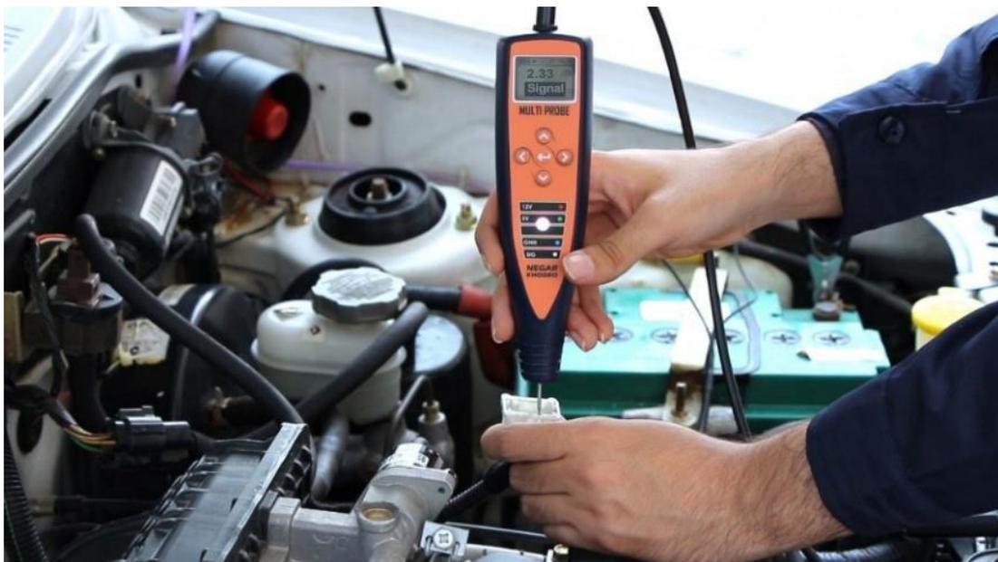
Gas valve sensor bases test
